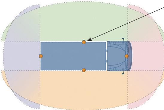
The four live images are simultaneously sent to an electronic control unit (ECU) where they are instantly processed, combined, blended, and stitched. The distortion from the wide-angle camera lens is also corrected before delivering a clear, single, smooth, real-time image onto the driver's monitor.
